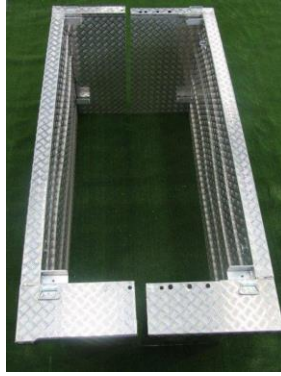
Showing shoring in 2 halves
