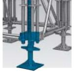
An extremely high loadbearing capacity is achieved by combining four Allround standards. A support of this type can be used as a single support (15 t load), as a double support (30 t load) or as a tower (60 t load).
