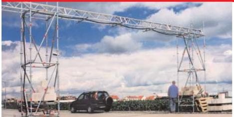
A simple and safe means for cross-overs are **bridging structures** made using Allround equipment: spans of up to around 12 m are quick to build using lattice girders, for any headroom required.
