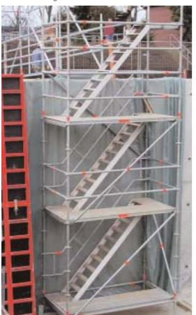
The Layher **compact stairway**, for example, puts an end to ad-hoc solutions in stairwells: flexible for every stairway opening and with minimum external dimensions of 1.55 x 1.75 m, it can be used for storey heights of up to 3 m.
