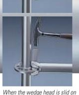
When the wedge head is slid on the rosette and the wedge is inserted into one of the holes, the part is immediately secured; a hammer blow on the wedge then creates an unbeatably strong connection.
