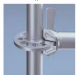
Speedy assembly is a built-in feature: the 4 narrow holes automatically centre the ledger at right angles — the 4 wide holes permit alignment of ledgers and diagonal braces at the angles required.
