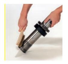
Simply remove the gasket ring once a year, loosen the safety screw, turn out the threaded part completely, clean and re-grease. Ready! Maintained this way, the spindle still turns freely after many civil engineering projects.
