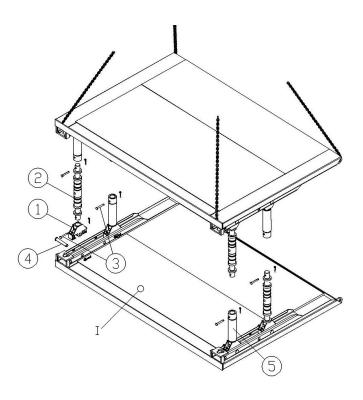
Lay the base plate on an even and solid surface with the post pointing upwards.
