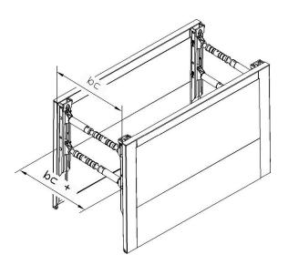
Now extend the spindles to the desired trench width (precision adjustment).
