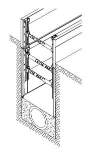
Once the pipe installation is completed, the shoring must be removed.
