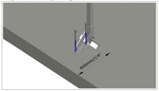
STEP 2: SCREW 2No.  $\emptyset$ M16 x 100mm /  $\emptyset$ 5%" x 4" BOLT (THUNDERBOLT OR EQUIVALENT) INTO HOLES AND ENSURE THEY ARE TIGHT.
