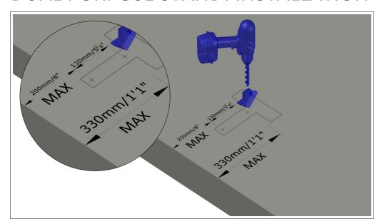
**STEP 1:** DRILL 2No. HOLES 115mm /  $4\frac{1}{2}$ " DEEP TO ACCEPT AN ØM16 x 100mm / Ø $\frac{5}{8}$ " x 4" BOLT (THUNDERBOLT OR EQUIVALENT), TO MANUFACTURERS SPECIFICATION.
