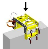
3. With the torque wrench, apply a torque of 25 to 30 lbf/ft to each of the eight bolts.
