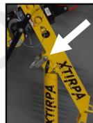
3. Remove the pin near the small pulley and rotate the semicircular bracket in order to pass the cable between the two pulleys. Once the cable is between the two pulleys, replace the pin and bracket so that the cable cannot slip out.
