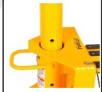
6. Lock the mast with the pin.
