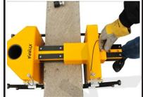
4. With the torque wrench, apply specific torque to each of the eight bolts.
