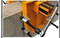
5. Insert the mast into the provided wing.
