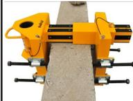
3. Adjust the removable part so that there is the smallest possible gap (less than 50 mm) for the bolts and lock with the pin.
