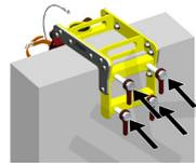
4. Insert the mast into the adapter.
